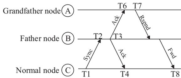
Fig. 4: Time synchronization model.
