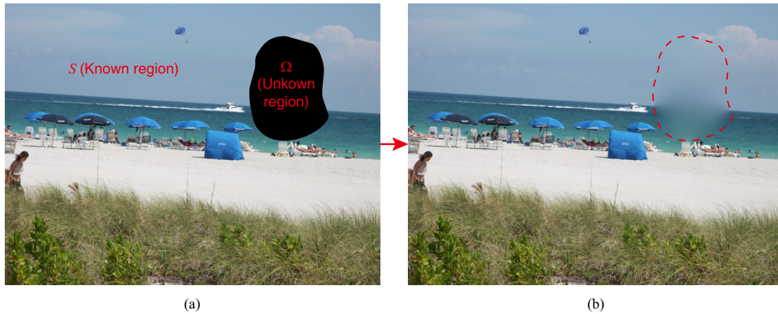
Fig. 1. An example of inpainting problem. (a) An image to be inpainted; the black region is unknown. (b) The inpainting result; the region surrounded by the dashed curve is recovered by inpainting.
